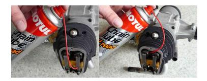
At the same time, or at least from time to time it is necessary to check the cleanliness of the motor, status / battery condition for ignition and the gap between the spark plug electrodes. This should be set **to 0.4 mm**. When the electrodes are burnt, replace the spark plug.
